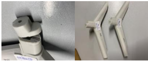
FACILAN C8 material, 30 % infill density
