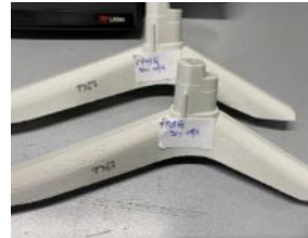
FACILAN C8 material, rPETG 30 % infill density
