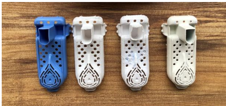
Left to right: original, 3D printed & unpolished, after testing 3D printed & unpolished, after testing 3D printed & polished
