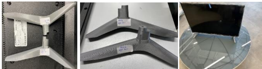
PETG material - with the infill density of 30 %, 15% and 20%.
